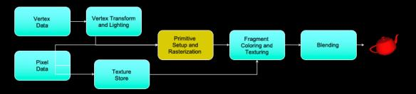
The initial version of OpenGL implemented a fixed-function pipeline, in which all the operations that OpenGL supported were fully-defined, and an application could only modify their operation by changing a set of input values (like colors or positions) through function calls. The other point of a fixed-function pipeline is that the order of operations was always the same – that is, you can't reorder the sequence operations occur.
