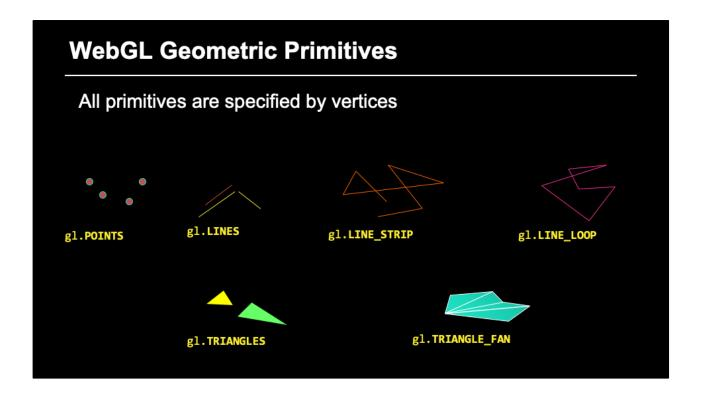
To form 3D geometric objects, you need to decompose them into geometric primitives that WebGL can draw. WebGL (and modern desktop OpenGL) only knows how to draw three things: points, lines, and triangles, but can use collections of the same type of primitive to optimize rendering.
