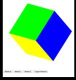
The next few slides will introduce our example program, one which simply displays a cube with different colors at each vertex. We aim for simplicity in this example, focusing on the WebGL techniques, and not on optimal performance. This example is animated with rotation about the three coordinate axes and interactive buttons that allow the user to change the axis of rotation and start or stop the rotation.
