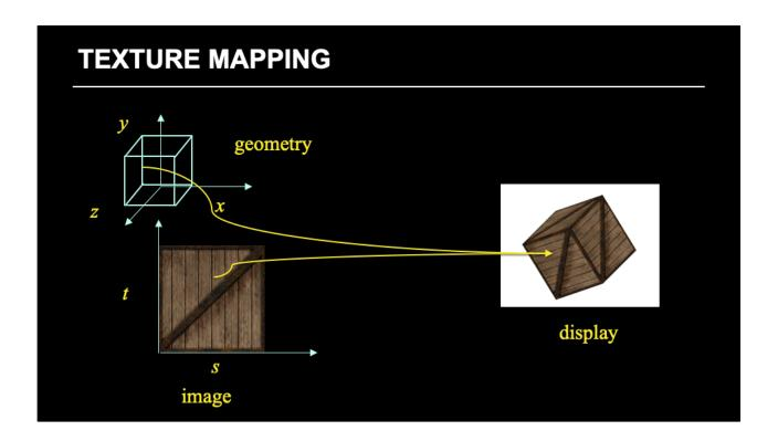
Textures are images that can be thought of as continuous and be one, two, three, or four dimensional. By convention, the coordinates of the image are s, t, t and t. Thus for the two dimensional image above, a point in the image is given by its t, t values with t0, t0 in the lower-left corner and t1, t1 in the top-right corner. A texture map for a two-dimensional geometric object in t2, t3 world coordinates maps a point in t3, t4 space to a corresponding point on the screen.
