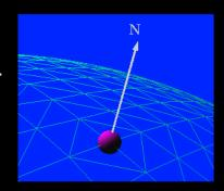
The lighting normal determines how the object reflects light around a vertex. If you imagine that there is a small mirror at the vertex, the lighting normal describes how the mirror is oriented, and consequently how light is reflected.
