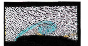
25. Visualization of 2D Velocity, Vorticity, and Deformation Rate Tensor
