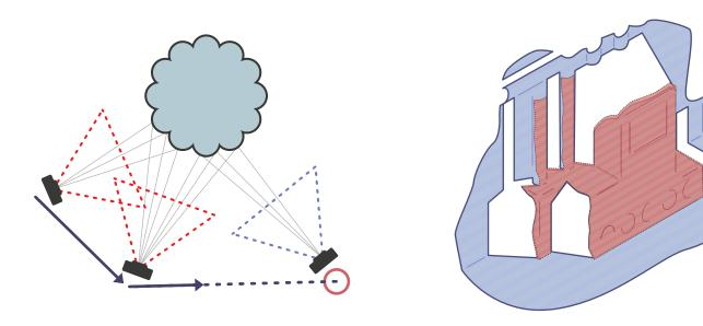
Using ORB (2D) and FPFH (3D) features, a number of estimations is made for all the different resources.
