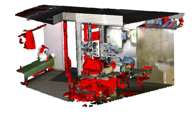
Remove all the points that both fail the coverage test (distance query) & the visibility check (normal comparison)
