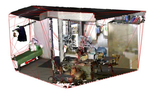
The convex hull of the XR dataset is used to query only relevant points.
