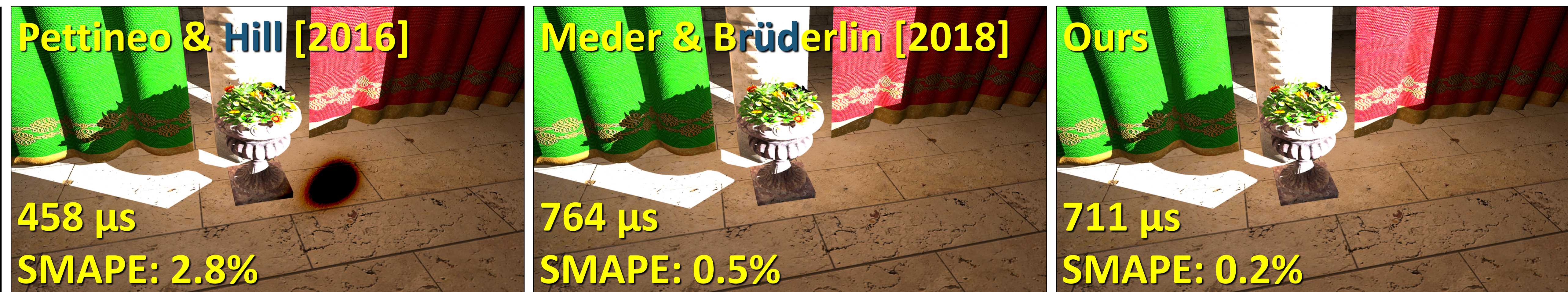
Dynamic indirect illumination using virtual SG lights [Tokuyoshi 2015]. Although Pettineo and Hill [2016]’s fitted irradiance is faster than Meder and Brüderlin [2018] and our method, it can produce undesirable black splotches. Our method does not produce such artifacts, and it is more accurate and slightly faster than Meder and Brüderlin.
