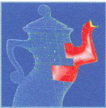
Tea Pot – Cyberware 3030RGB/MS Scanner . Multiple scans combined into point cloud. Shown is creation of NURBS surface using Imageware's Surfacer.
