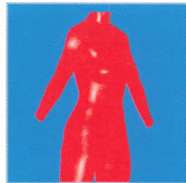
NURBS Nude – Live subject. Cyberware WB4 Body Scanner . NURBS surface from point cloud. Surfacer software.
