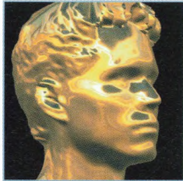
Jason's Head – Live subject. Cyberware 3030RGB/PS Scanner . Converted to DXF. Smoothed and rendered in 3D Studio. 15 minutes.
