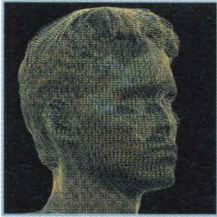
Jason's Head – Live subject. Cyberware 3030RGB/PS Scanner . Converted to DXF. Smoothed and rendered in 3D Studio. 15 minutes.
