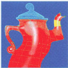
Tea Pot – Cyberware 3030RGB/MS Scanner . Multiple scans combined into point cloud. Shown is creation of NURBS surface using Imageware's Surfacer.
