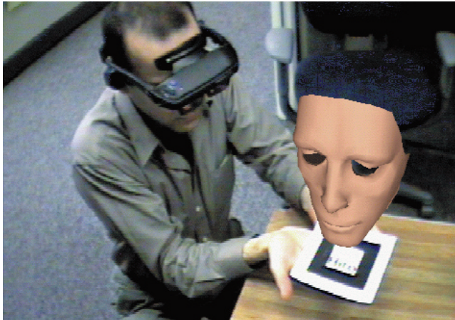
The view through the head-mounted display in a face-to-face setting. Users can see their collaborators and virtual objects between them.
