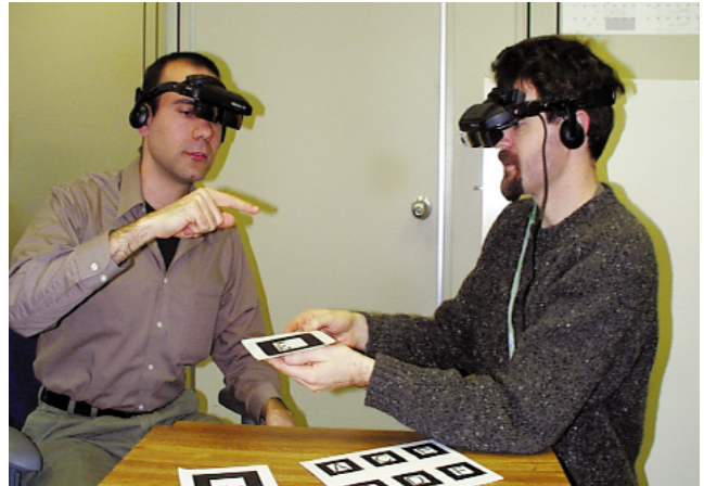
View from outside the interface. The virtual objects are only visible to those wearing the head-mounted displays.
