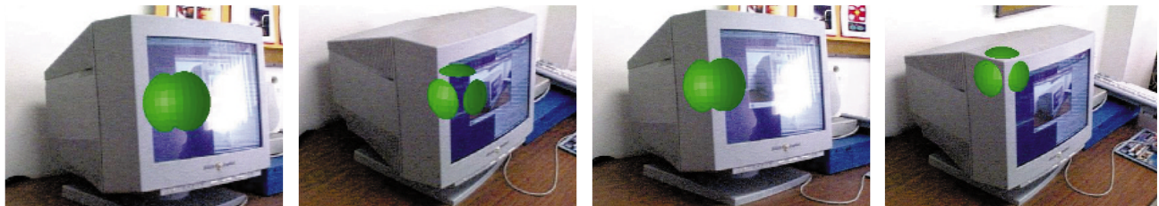
Figure 2 Misalignment of real and virtual objects (left), and correct registration after error compensation (right).
