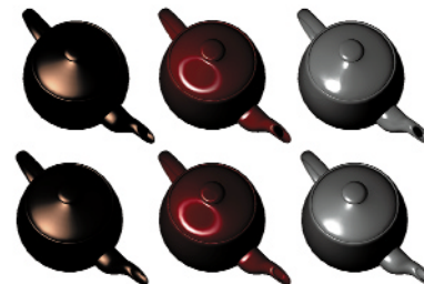
Figure 1: Left to right: HTSG copper, Ward's anisotropic model, and measured grey vinyl. Top: Models with BRDFs evaluated at every pixel in a raytracer. Bottom: Hardware-accelerated single-term approximations using OpenGL.
