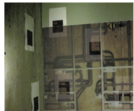
Augmented reality X-ray view inside a wall for building maintenance personnel. (Courtesy of Fraunhofer Institute for Computer Graphics)
