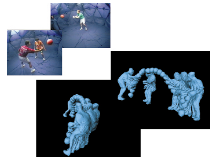
An input sequence is digitized into a Virtualized Reality 4D event model. (Carnegie Mellon University)
