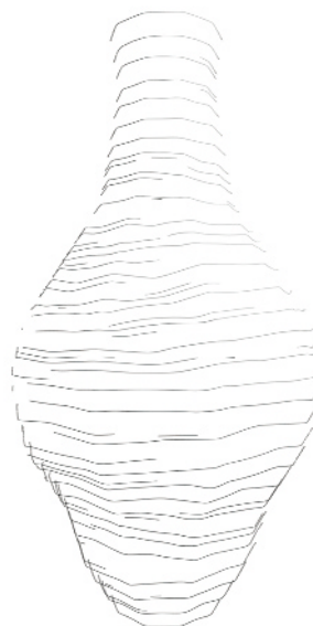
Figure 2 Principal direction line drawing of a vase. Mesh consists of 400 triangles.
