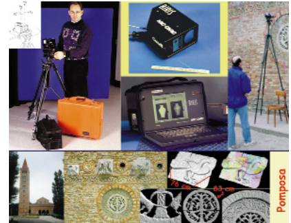
Figure 1 Top and center: portable 3D imaging system includes a Biris camera (standoff: 30 cm, range: 200 cm, data rate: 15,360 3D samples per sec, weight: 900 gr.), a pan unit and a tripod. Bottom: outdoor application at the Abbey of Pomposa (circa 850) in Italy 1998.
