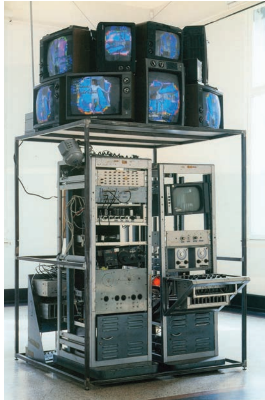
Figure 5. The Paik-Abe Video Synthesizer (PAVS), 1969 / 92. 183 x 56 x 66 cm. 12 monitors, two video disc players. Image courtesy of Paik Studios/Nam June Paik Estate. © 1992 Nam June Paik and Shuya Abe.
