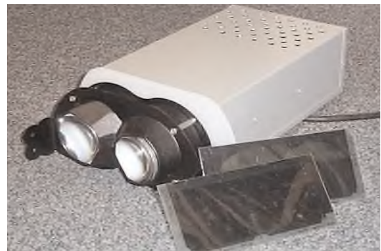
Figure 1: HDR Viewer capable of 10,000:1 contrast ratio.
