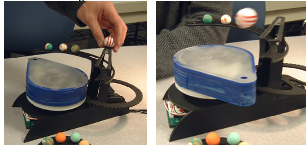
Fig. 2. The ball rolls down the ramp and an air stream levitates it.
