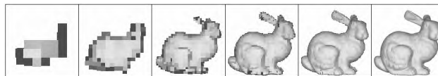
Figure 2: A sequence of progressively refined, splatted volumetric models. Each finer model contains and covers all coarser models.
