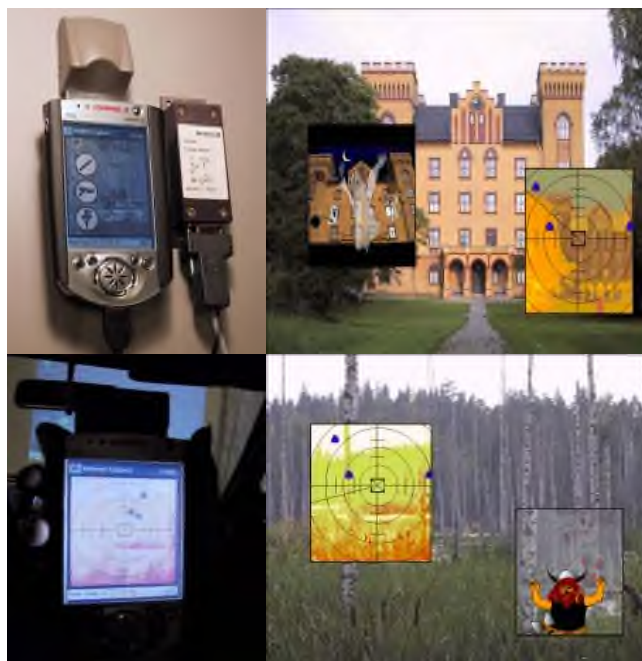
Figure: From top left moving clockwise. 1. Pocket PC with GPS and digital compass. 2. The castle with the ghosts overlayed. 3. The swamp with the viking and the ghosts overlayed. 4. The test environment for the game, with the targeting functioning.
