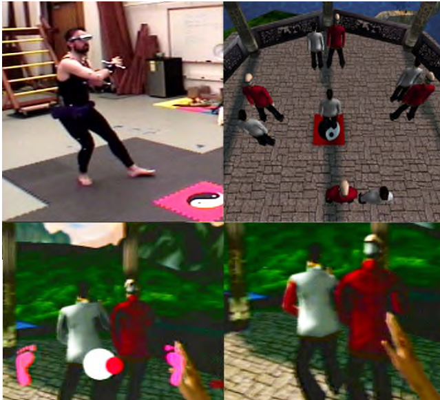
Figure 1: Top-left to bottom-right: A student in the trainer. The virtual world. Center of gravity display. Coloring the limb with the largest error
