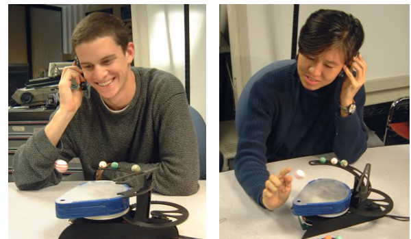
Fig. 3. In conversation: the ball floats up and down in correspondence to the remote person’s movement.
