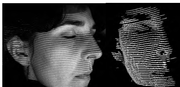
Figure 2. Laser raster projected onto a person's face (left). 3D reconstruction of the lines (right).
