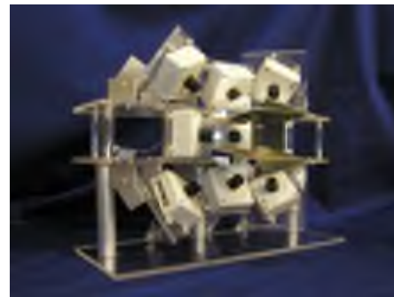
Figure 2. Camera-head with nine video cameras
