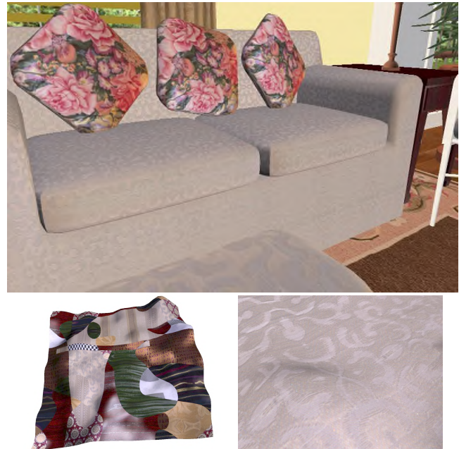
Figure 1. Real-time rendered SBRDF scenes. Top: Measured couch fabric, curtain, and plant leaf SBRDFs; synthetic wood and brass SBRDFs. 260,000 polygons, 3 lights, 57 frames / second on Nvidia GeForce 4. Bottom: Left: One texture map with 2^{20} different BRDFs. Right: Fabric shows subtle shading changes due to variation in thread material and direction of anisotropy.
