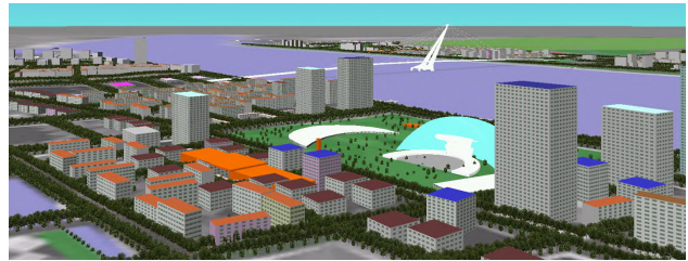
Figure 2: Custom CAD models (Opera house and bridge) and buildings procedurally generated from GIS attributes. Roof colors represent land use type.
