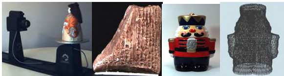
Figure 1: (from left to right) Zoomage3D scanning device, a tiny 3x2 sq.in. stone with writing on it, a 1 ft tall nut-cracker toy and a 18,720 polygon wireframe of the toy.
