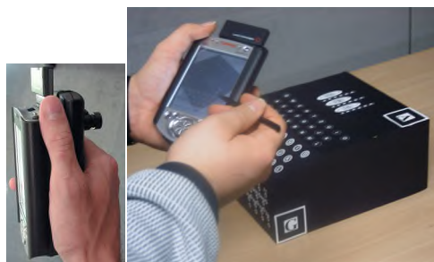
Test Setup: PDA with Camera, WLAN card, video up-link and Enigma Mock-up
