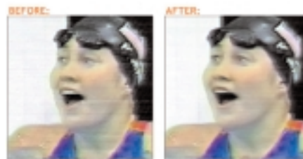
By combining the data over frames, VideoFOCUS can produce an image with less noise and higher overall resolution than any individual frame.
