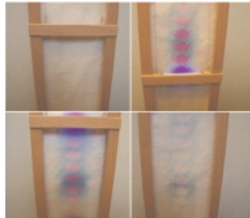
Figure 1. A textile is mounted in a wooden rack, and a computer-controlled motor moves a UV lamp over the fabric to create different patterns. The color changes remain visible for 5-10 minutes after the last UV exposure.
