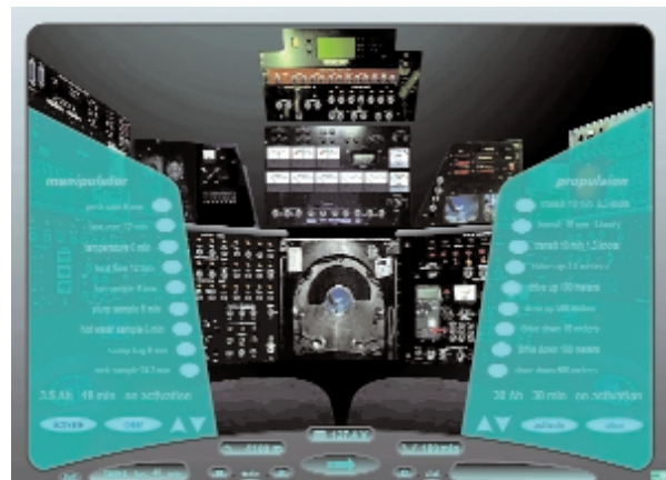
Figure 1. Virtual ALVIN mock-up (upper left) and final Web-based simulator interface in Flash. 3
