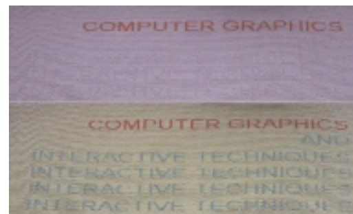
Figure 2. The top image shows another custom-created textile in its initial state; the bottom image shows it after it has been subjected to UV light, revealing additional text woven into the fabric. (The background has also changed color.) The new text remains visible for 5-10 minutes after the UV light has been removed.
