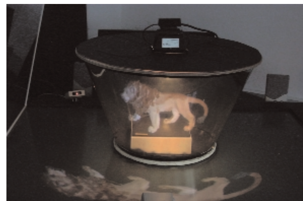
Figure 1. Two different Virtual Showcase configurations: a truncated pyramid (top) and a cone-shaped device (middle/bottom).
