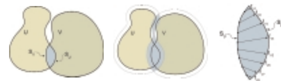
Figure 1. (a) The overlap region (in blue) of shapes U and V is determined by local generation of the intersection of U and V; (b) the overlap region of the offset surfaces of U and V can also be easily generated for determining proximity information; (c) forces acting on S_V in the overlap region of (a).
