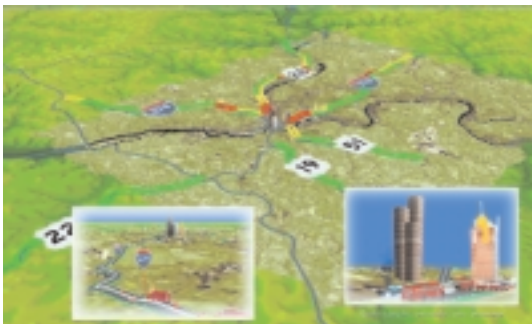
Figure 1. Virtual world used to produce animated road traffic reports for a particular metropolitan area. Colored segments overlaid on major highways indicate traffic conditions.
