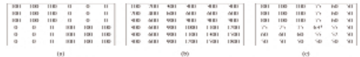
Figure 1. From texture (a) to summed area table (b) to averaged area able (c).
