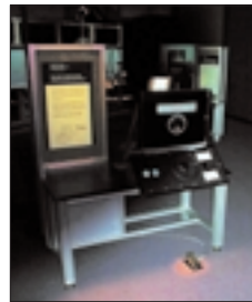
Figure 2. Presentation graphics and physical overlay for Speeder Reader. Blue indicates the side-lit laser-cut Lexan overlay; red and black, and the background to the text, are all screen display areas; white shows where physical layers of felt and black plastic (under the top-layer Lexan) block the rest of the computer monitor from view.
