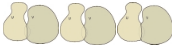
Figure 2. Contact deformation of the objects of Figure 1 with (a) similar material densities; (b) V softer than U; and (c) volume preserving deformation. 7,8
