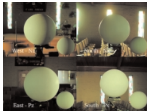
Comparison test with rendered diffuse ball from HDR fisheye environment maps composited over photographs of matte-painted beach ball.
