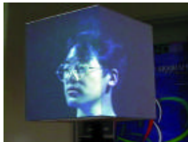
Projected image. Both the image and the cubic screen are controlled to follow the remote person's head motion.
