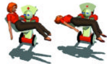
Figure 3: Nursing care robot with special consideration of how forces can be applied to a patient
