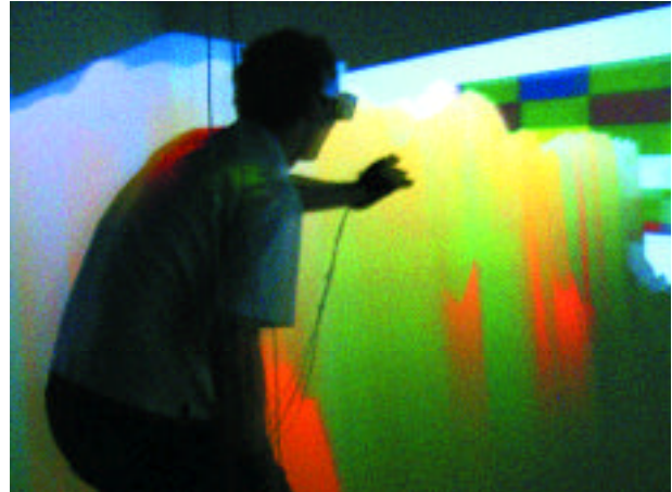
Figure 4: A researcher uses a pinching motion to warp the height field, in this case making a pale blue area more saturated by drawing it upward.
