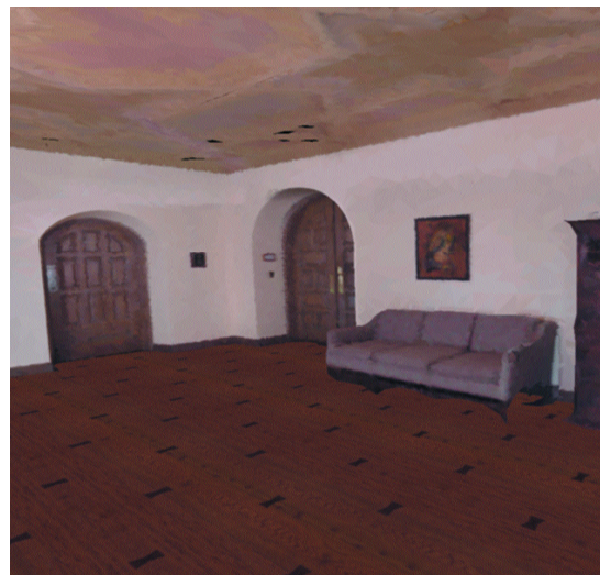
This second image shows the same room rendered with only five texture maps produced from clustering.
