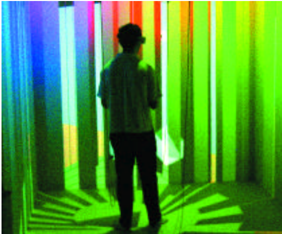
Figure 3: Ribbons help to convey the location of colors in an HSL cylinder without obstructing the user's views of the space.
