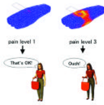
Figure 2: Prediction of Pain Level in Using Bag (by the result of equivalent strain value on the forearm)
