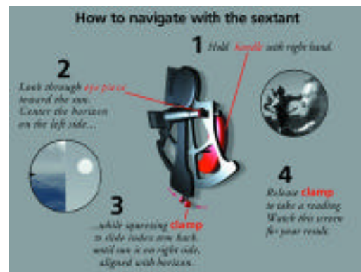
Screenshot from navigation interactive shows the startup state of the LCD screen. A real sextant is the only input device, and when a visitor manipulates it, the screen responds accordingly.
