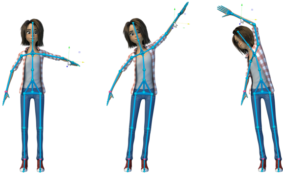
Fig. 8. The user is manipulating the character’s left arm for a static pose. The feet and right hand are pinned, ensuring that they do not move during manipulations.
