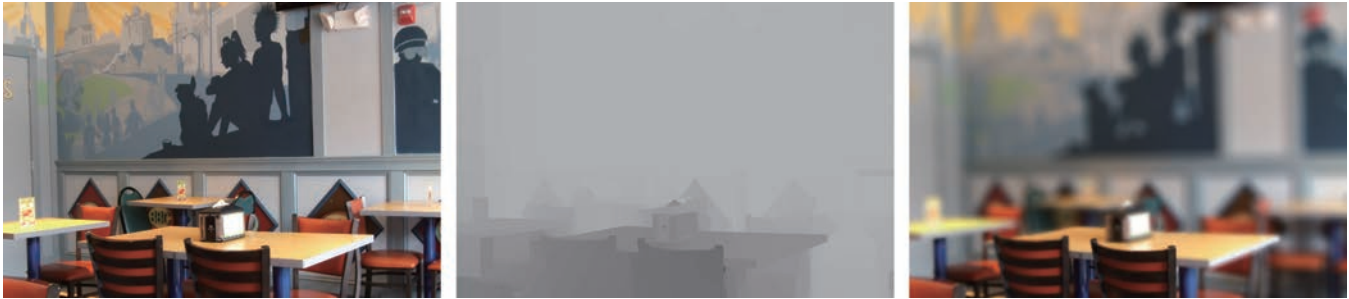
Figure 1: Left: The left image captured from a stereoscopic camera. Middle: The estimated depth map. The dark color indicates the pixel is close to the camera. Right: The synthesized image, in which the focus is at the chair.
