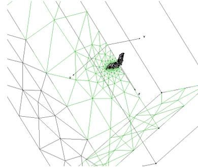
Figure 2: A user specifies, in Gridgen, which surfaces should be triangulated.
