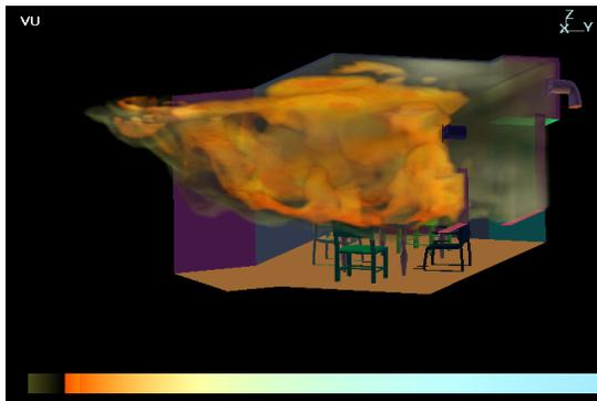
Figure 1: A Fully Developed Backdraft.
