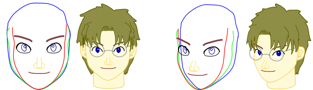
Figure 3: A sample of a composite 3D outline. If viewed from in front of the face, the blue outline is rendered. (Left) On changing the viewpoint, the red and green outlines are partially rendered. (Right)
