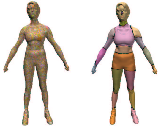
Figure 1: This model has 141,837 notches. Left: Exact convex surface decomposition – 44,461 components. Right: Approximate convex surface decomposition – 20 components (concavity < 0.05 ).
