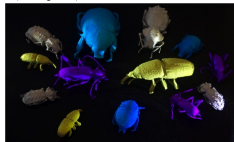
Figure 2. Insect models, 3D printed in titanium.
