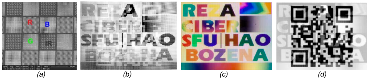
Figure 1: The Nano-Media concept (a) SEM image of the pixelated substrate (b) Microscopic image of the ICL (c) Full color images displayed by the Nano-Media after aligning (a) and (b) taken by a camera (d) Covert QR Code stored on the Nano-Media and is read by a camera using an IR edge-pass filter (Inverted).
