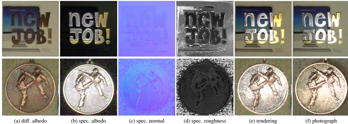
**Figure 1:** Reflectance properties of flat samples acquired using a mobile device. Top-row: Hand held back camera-flash pair acquisition for rough specular BRDFs. Bottom-row: Tablet based acquisition using front camera and LCD screen illumination for highly specular BRDFs.
