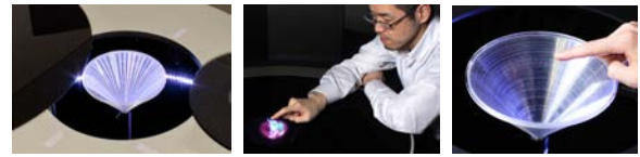
Figure 1: Projector array (dots seen from opened hatch) and hollow conical screen covered by semi-transparent plate.
