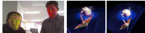
Figure 2: Adaptive vertical-perspective correction. Results of face detection and 3D images for two different viewing heights.
