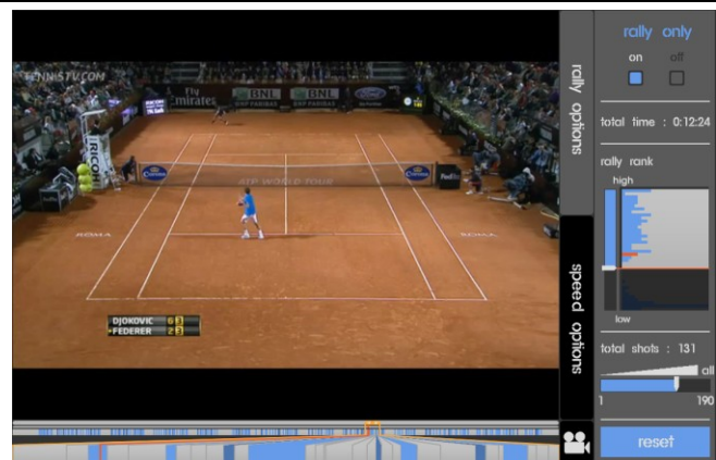
Figure 1: User interface for racquet sports video. Bottom: time bar indicating shots. Right: viewing method settings (rally options, speed options).
