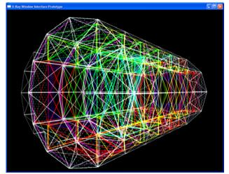
Figure 1. X-Ray Window Rendering of ISS *Destiny* Module, with Color-Coded Stowage and Equipment Components
