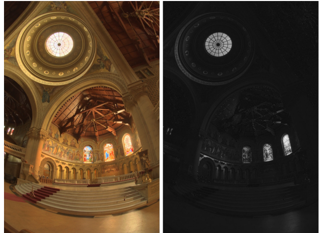
Figure 3. Memorial Church tone-mapped with Reinhard’s global operator next to ratio image needed for HDR recovery. (Image courtesy Paul Debevec.)
