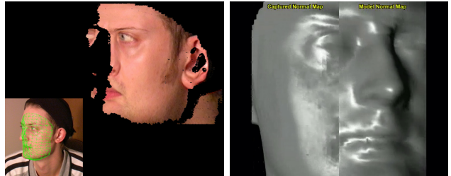
Tracking: The head position is tracked, and the video image unwrapped into texture coordinates, simulating a moving light source and fixed head.
