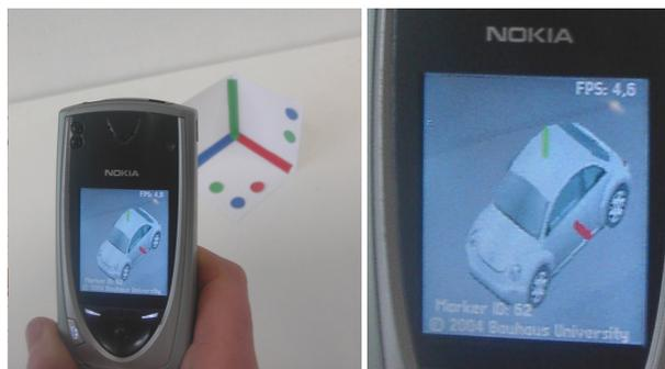
Figure 1: 3D graphics rendered perspectively correct into the live video stream with respect to the position of the cell phone relative to the marker.
