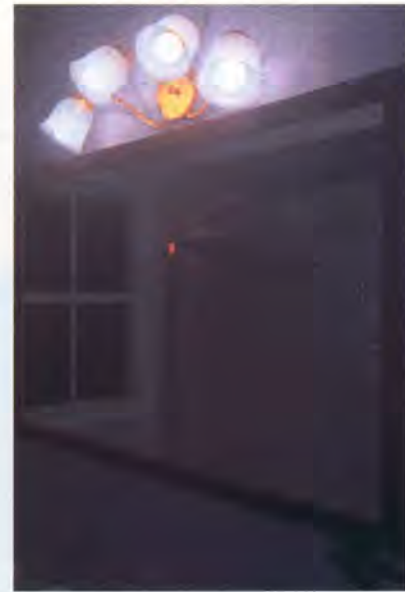
FIGURE 3 The same simulation reproduced using the new tone mapping operator, which models human contrast sensitivity and disability glare.
