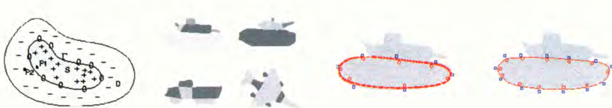
FIGURE 2 Parts database for object shapes and indexing based on the tank body part
