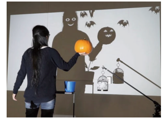
(b) Deforming real shadows by projecting virtual light sources inside the real shadows.
