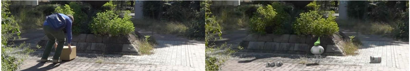
Figure 1: Shooting video on the left; the same shot with reconstructed z depth and 3D real-time elements on the right.
