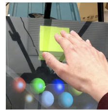
Figure 5: Moving a mid-air 3DCG object by hand.
