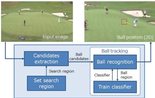
Figure 3: Process flow of ball tracking module.
