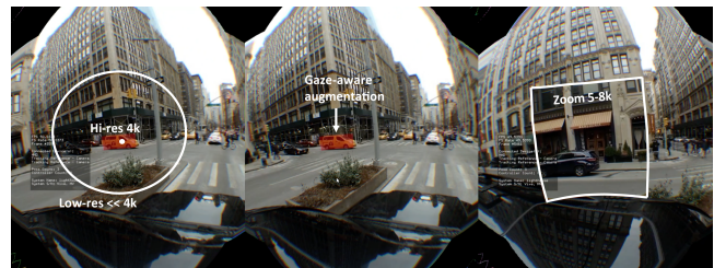
Figure 1: From left to right, a) foveated composition and b) foveated augmentation, and c) new display modalities for increased immersivity, e.g. 5-8K Zooming
