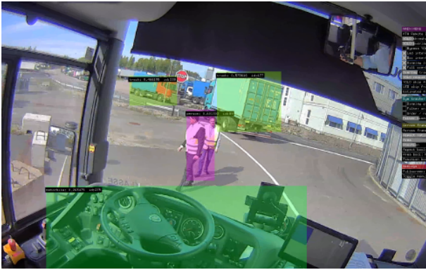
Figure 2: Example of task-aware augmentations inserted for supporting a remote driving task.
