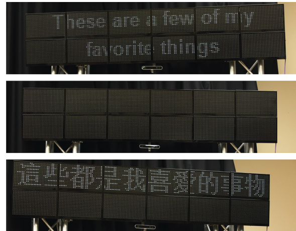
Figure 3: A PARALLEL REALITY™ display as seen from 3 different view points. Note that each view can see a different language of captioning or no captioning at all.
