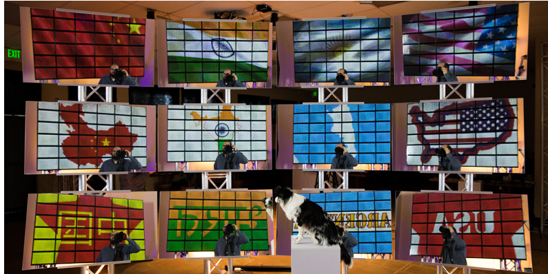
Figure 1: A single PARALLEL REALITY™ display as seen reflected in a dozen mirrors. Note that each mirror is reflecting what an individual at the mirror's location would see when looking at the display.
