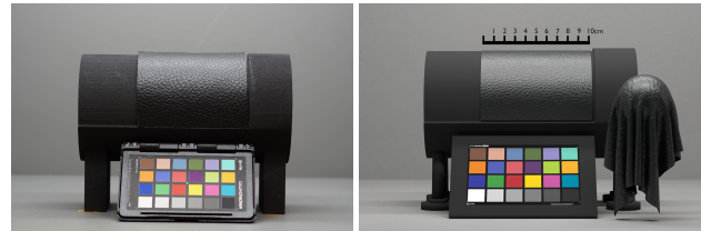
Figure 2: Lightbox setup for material creation: reference photo and corresponding (rendered) material creator view.
