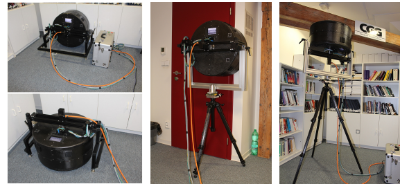
Figure 2: Measurement on site (left) floor based holder for floor and wall close above the floor, (middle) tripod based holder for measuring on a wall and (right) for measuring on a ceiling.
