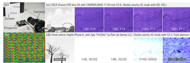
Figure 3: (a) Setup for evaluation from camera vision. (b) Images are divided into three parts. Projection period (see Figure 1) is 4166 microseconds (approximately 240 Hz). (c), (d) Images from camera vision. Please note that f-stop of smartphones is fixed (specification).
