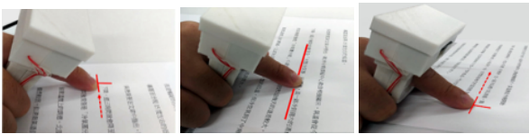
Figure 3: Haptic feedback mechanism of guidance reading mode. (a) Guidance to the start of line, (b) Skipped line notification, (c) End-of-line notification.
