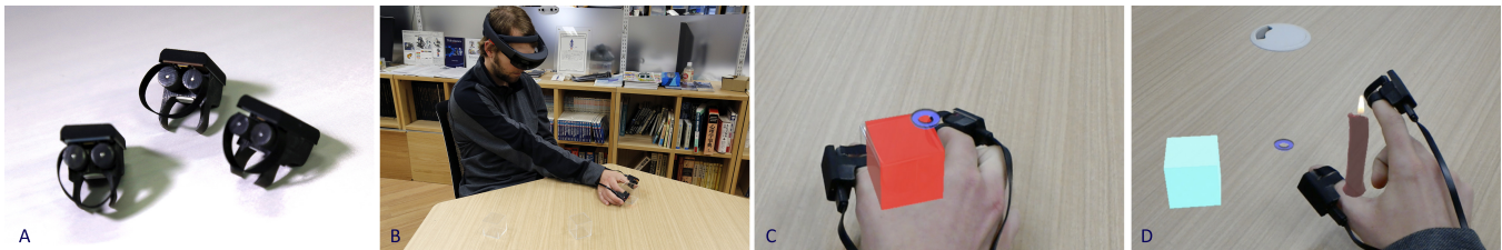
Figure 1: (a) Augmented Haptics Display, (b, c) Touching a haptic augmented clear cube, (d) Augmented thermal cues
