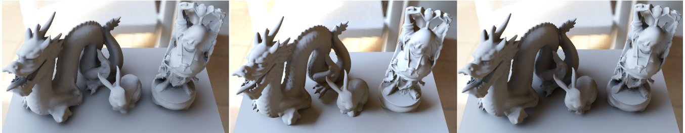
Figure 1: Left: Irradiance map with bent normal + AO (8.0 ms). Middle: Raytraced ground truth. Right: Our approach (7.2 ms).
