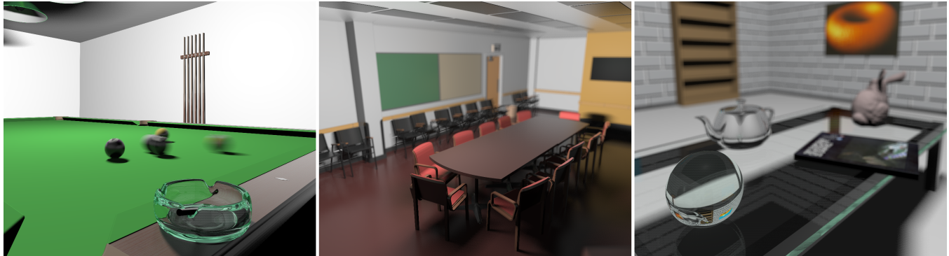
Figure 1: Ray tracing can robustly and naturally support next generation visual effects not easily combined with GPU graphics including depth-of-field, motion blur, glossy and specular reflection, soft shadows, and correct refraction. More details on the system that generated of these images are available in Boulos et al. (2006).
