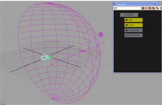
Figure 1. Stereo camera rig showing left and right cameras, zone of exclusion and point of parallax.
