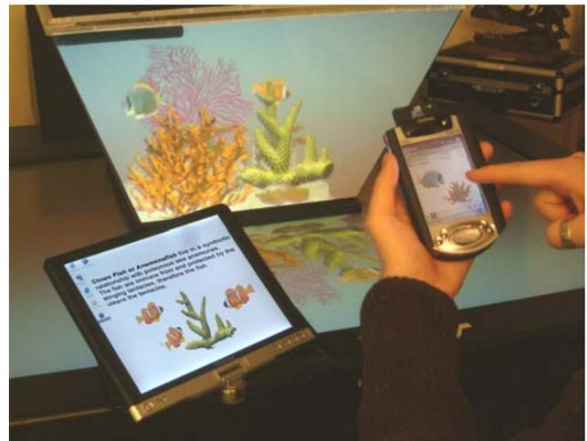
**Figure 2: An example configuration of the Interactive Aquarium systems showing all three components. Towards the back is the Virtual Aquarium, to the left the stationary interaction and being held, the mobile interaction panel.**
