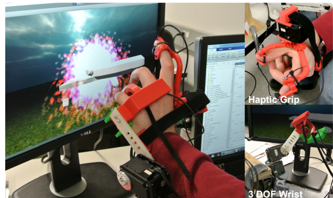
Figure 2: An exoskeleton with admittance-controlled 3-degrees-of-freedom wrist and a finger/thumb grip haptically interacting with virtual objects in a 3-D animated environment.
