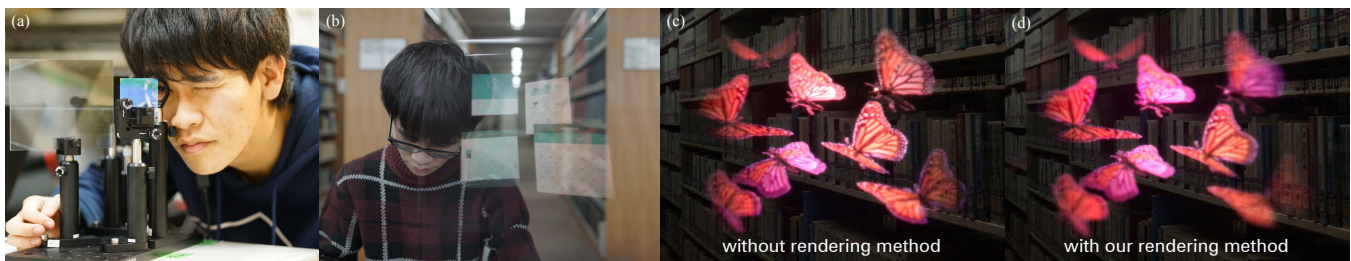
Figure 1: (a) Prototype display based on our optical schematics. (b) The obtained image from see-through prototype. (c), (d) The result of applying simulated retinal blur. Note that there is a difference between the image acquired by the camera and the image actually seen through the human eye.
