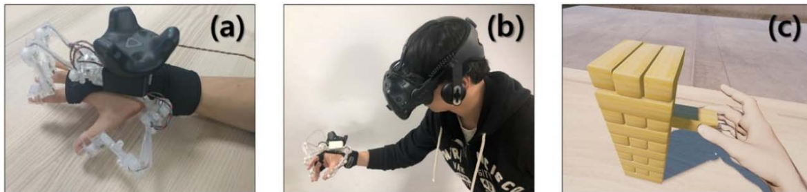
Figure 1: (a) CHICAP, hand motion capture device. (b) Hand operation using CHICAP in real world. (c) Corresponding object manipulation in virtual world.
