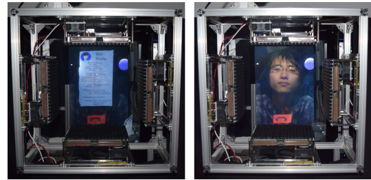
Figure 5: Left: interface screen is superimposed onto the opposite user's face. Right: a main part of screen's brightness is at its lowest level.
