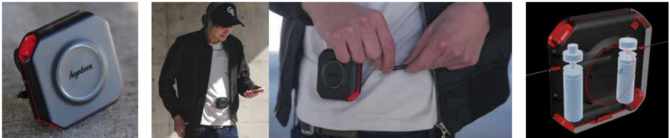
Figure 1: Left: The Hapbeat, Middle: How the device is worn, Right: Internal structure
