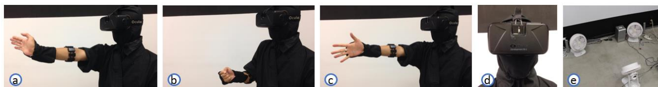
Figure 1: We propose a method to allow the user to move around in a virtual space without walking. By combining several wearable devices and a wind-feedback system, we provide the user a new experience of exploring 3D space. More specifically, a user can (a) throw his wrist to shoot the spider silk, (b) grab and pull the silk to move forward, and then (c) release the silk for the next move. Here, (d) the IMU in the HMD is used to detect the jumping events, and (e) the wind-feedback system is adopted to enhance the feeling of moving.
