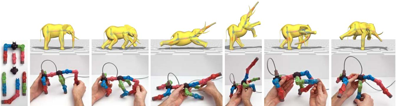
**Figure 1:** Assembled from modular, interchangeable, and hot-pluggable parts (left), our novel device forms a skeletal tree matching the Elephant. As the user manipulates each joint of the device, measured bone rotations animate a skeletal rig, and the Elephant comes to life.
