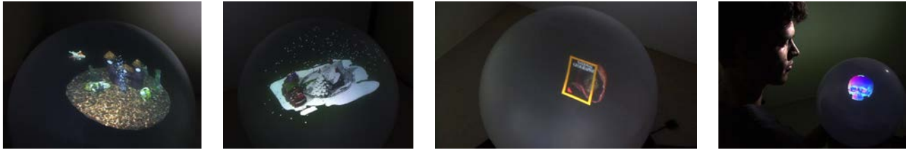
Figure 1: Spheree is an interactive spherical rear-projected display that provides perspective-corrected views (based on the user's head position) to provide parallax, perspective, shading and occlusion depth cues.
