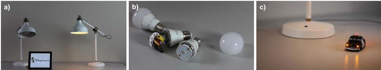
Figure 1. a) Demo setup with off-the-shelf lamps, b) modified consumer light bulbs, c) toy car equipped with VLC technology
